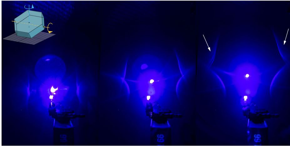
Fig. 3. Artificial Lowitz arcs (Ref. 13) generated by the mounted and spinning module in Fig. 1(a) with increasing light source inclinations ( 0^\circ – 30^\circ ). A low-power, focusable, blue laser diode ( \lambda = 405 nm, P < 1 mW) was used for illumination. The arrows indicate a faint feature/arcs appearing distinctly only at large elevations (Ref. 13).
